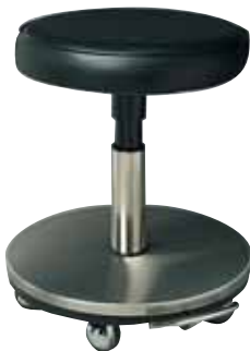
Model 3881151 Surgeon Stool: Foot operated, black vinyl upholstered circular stool. Height adjustable between 530 - 710mm by foot operated mechanism.
