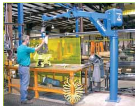
Easy Arm - an articulated jib crane with an in-built G-Force™ end effector.
