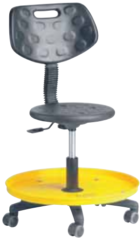
Model 3721057 Universal Stool: Black PU circular seat with ring lever underseat mechanism, black PU backrest 545mmØ yellow powder coated dish attached to a 5 leg nylon base. 50mmØ soft grey rubber castors - 2 locking, 3 free rolling.
