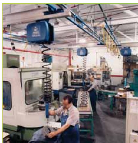
Easy Arm - an articulated jib crane with an in-built G-Force™ end effector.
